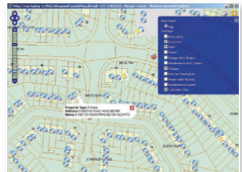
Events, customer calls, network assets, and properties can be displayed on the spatial viewer to aid fault and incident assessment
