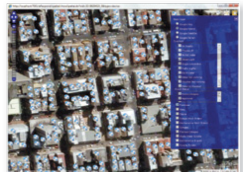
Network Events, Customer Calls, Network Assets, and Properties can be displayed on the spatial viewer to aid fault and incident assessment
